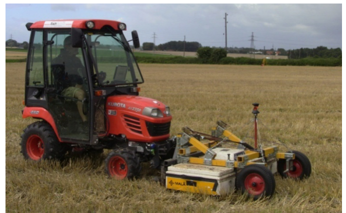
Figure 2. GPR measurements with the 16 channel 400 MHz MALÅ Imaging Radar Array (MIRA) with 8 cm channel spacing using a total station visible in the background together with a prism for automated data positioning.
