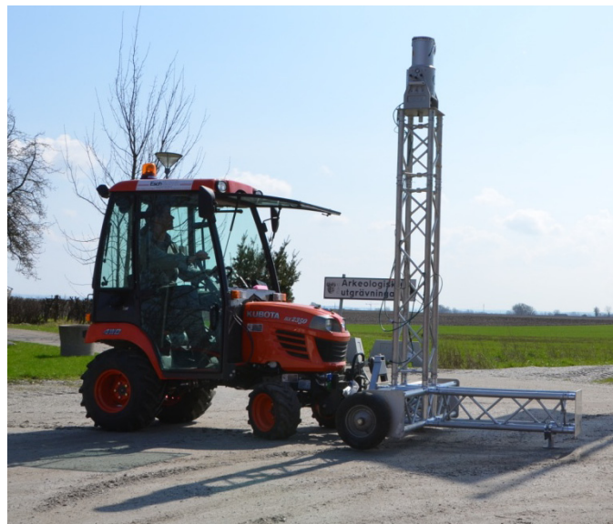
Figure 4. Laser scanning for the generation of a high resolution terrain model using a Riegl LMS-Z420i scanner mounted on top of a tripod, between scanning positions is transported with a small tractor.
