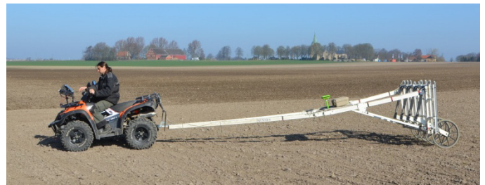
Figure 1. Magnetic survey with motorized 10-channel Foerster gradiometer array mounted with 25 cm probe spacing on Sensys cart in April 2011. The RTK-GPS antenna for data positioning is visible on the cart. Data logging and navigation is implemented using custom software on a rugged laptop in front of the operator. In the background Uppåkra church can be seen.
